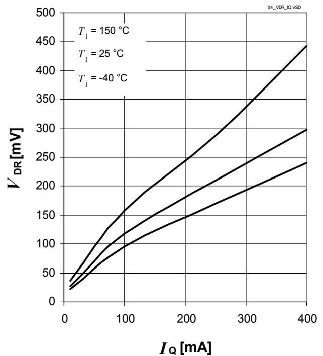
**Dropout Voltage  $V_{dr}$  versus Junction Temperature**
